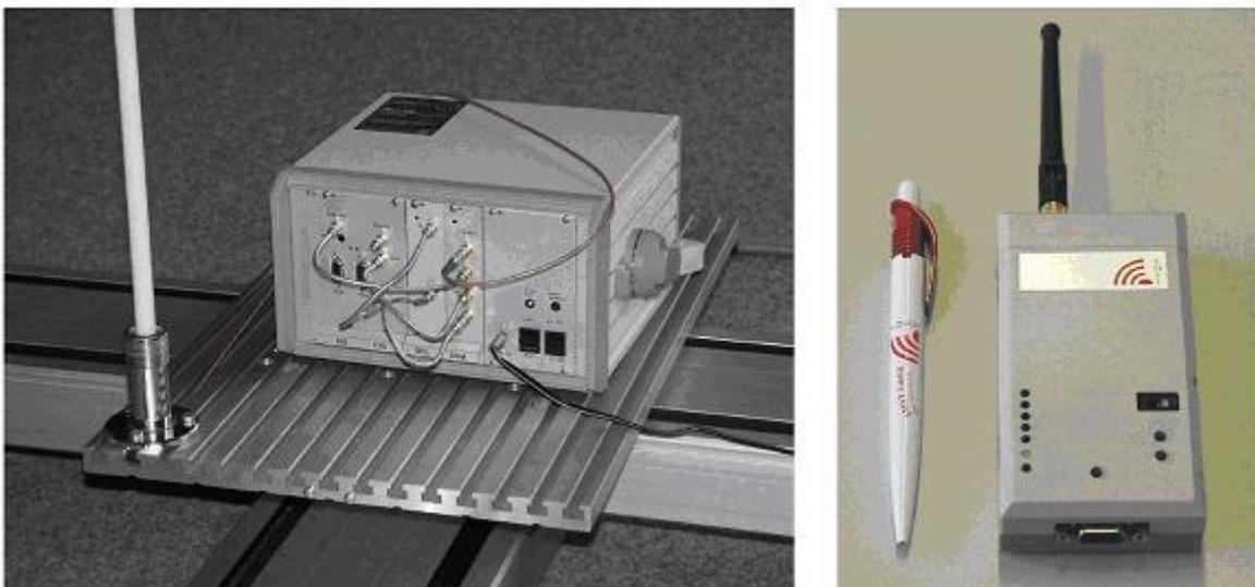
Figure 82: Iltis mobile stations from IMST: 1<sup>st</sup> generation (left) and 2<sup>nd</sup> generation (right) [76]
