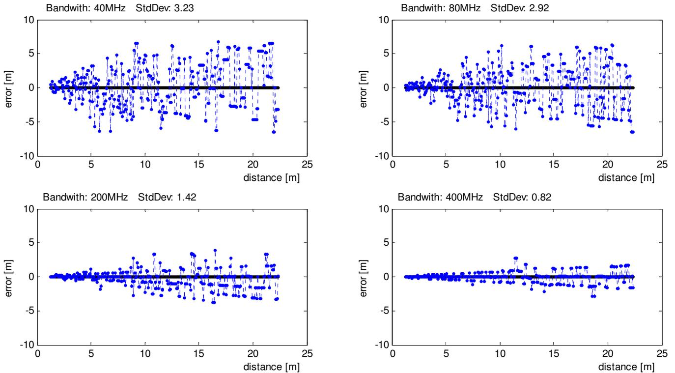
**Figure 77: Estimation error of the VRU position relative to the road using triangulation with an obstacle**
