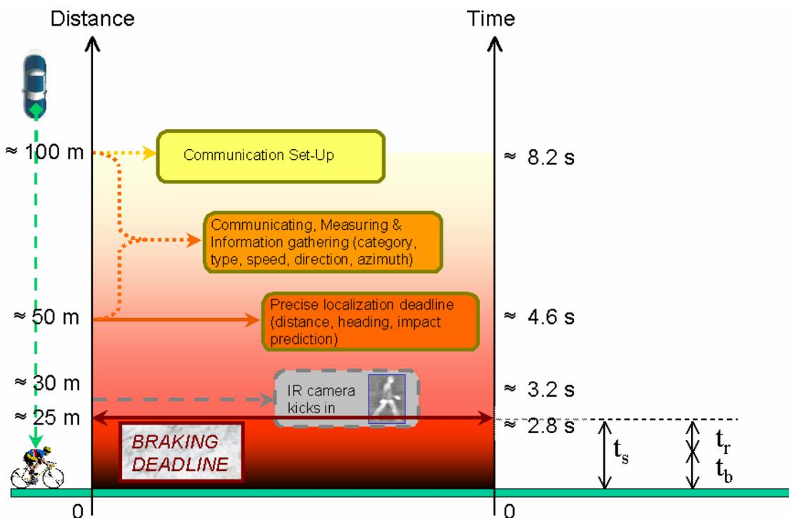
**Figure 1: Basic Timeline and Distances for the Localisation System**
