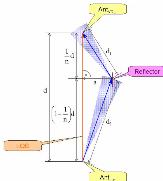
**Figure 5: Detour of the signal because of NLOS propagation conditions**
