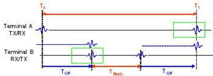
**Figure 65: Asymmetric Two Way Ranging [19]**
