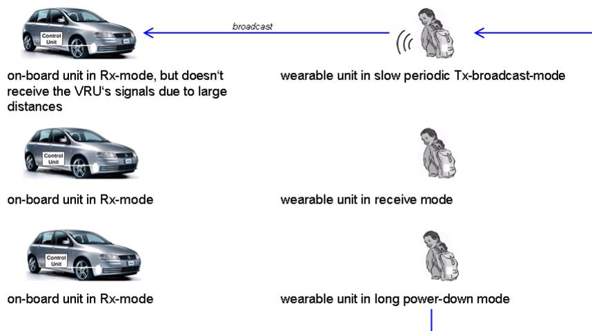
**Figure 9: Initial state of communication between wearable and on-board unit**
