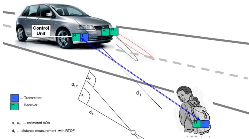
**Figure 69: Angle-of-arrival (AOA) based approach with two estimation methods
