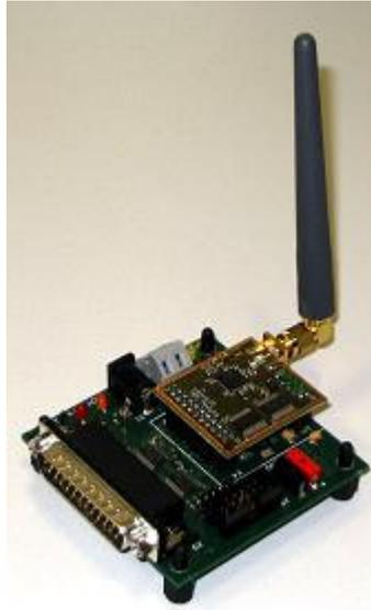
Fig. 2: nanoLOC ASIC Ranging Demonstrator components
