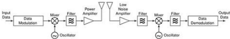
Figure 51: A typical narrowband transceiver architecture [36]
