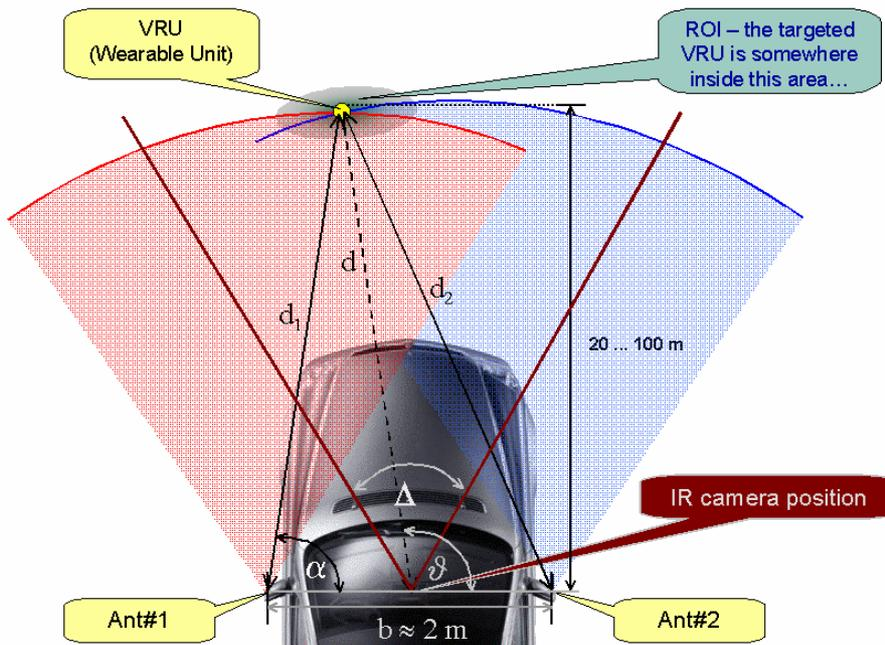
**Figure 2: Arrangement of the localisation system, distance measurement approach**
