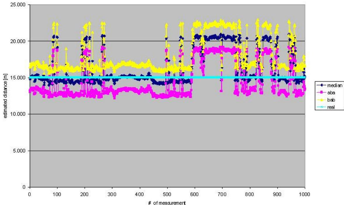
Fig. 14: Measurements with a significant number of deviating results; point a1, point b2 at a distance of 15 m (raw results)
