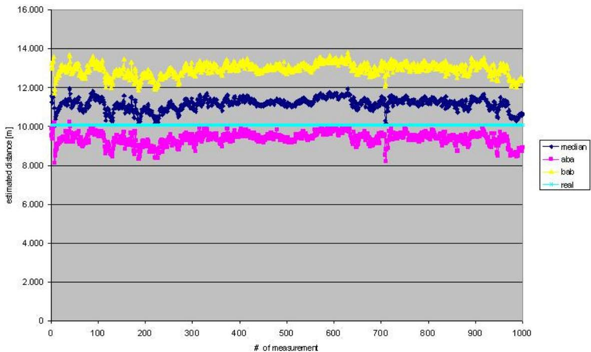
Fig. 13: Measurements with single deviating results; point a3, point b2 at a distance of 10 m
