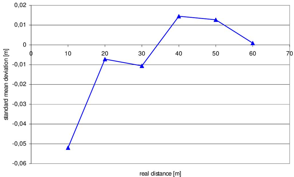
Fig. 32: Standard mean deviation for static measurements without obstacles in setup 2 using the nanoLOC ASIC
