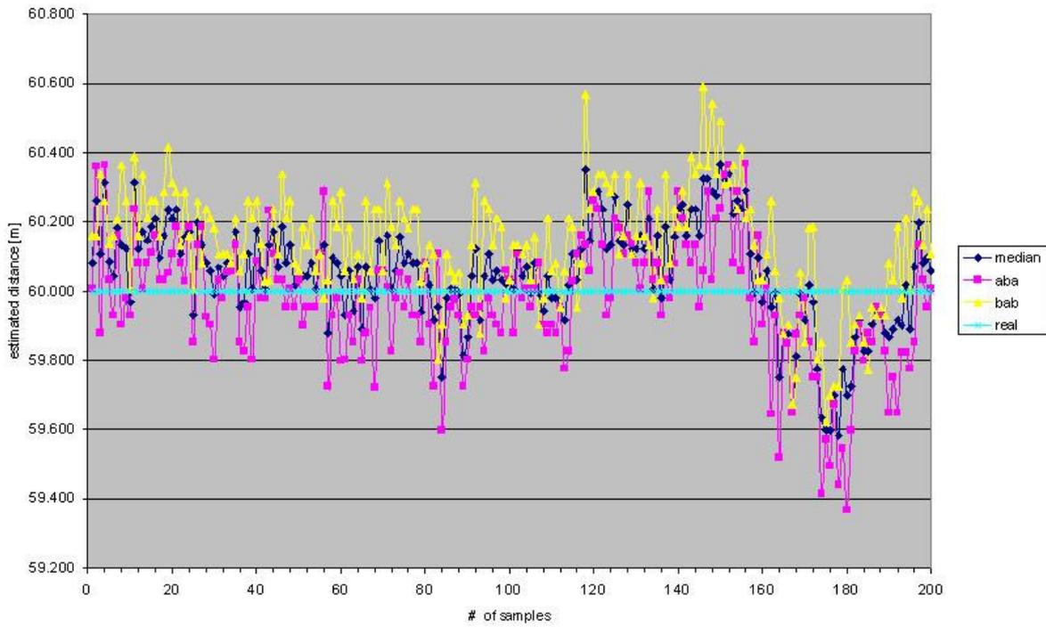
Fig. 30: Estimated distances for 200 samples using the nanoLOC ASIC; real distance is 60 m
