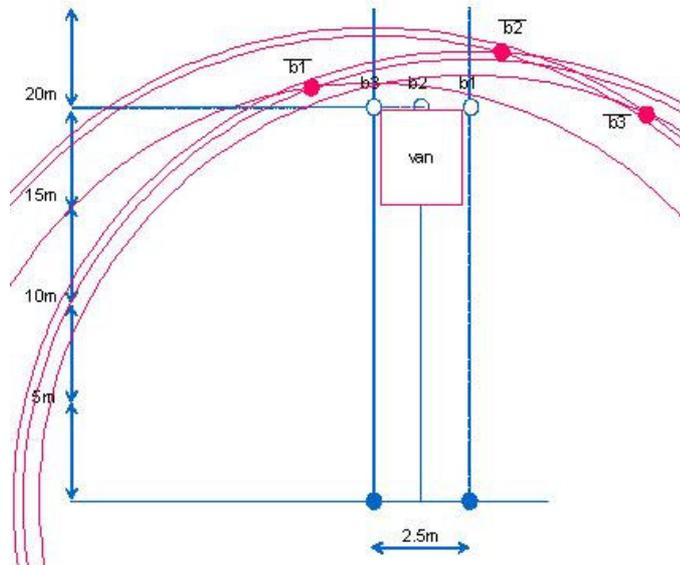
Fig. 21: Illustration of measurement results for test setup 1 with a van parking at the 15 m line. The circles show the diameter of the measured distances from both points a1 and a3.
