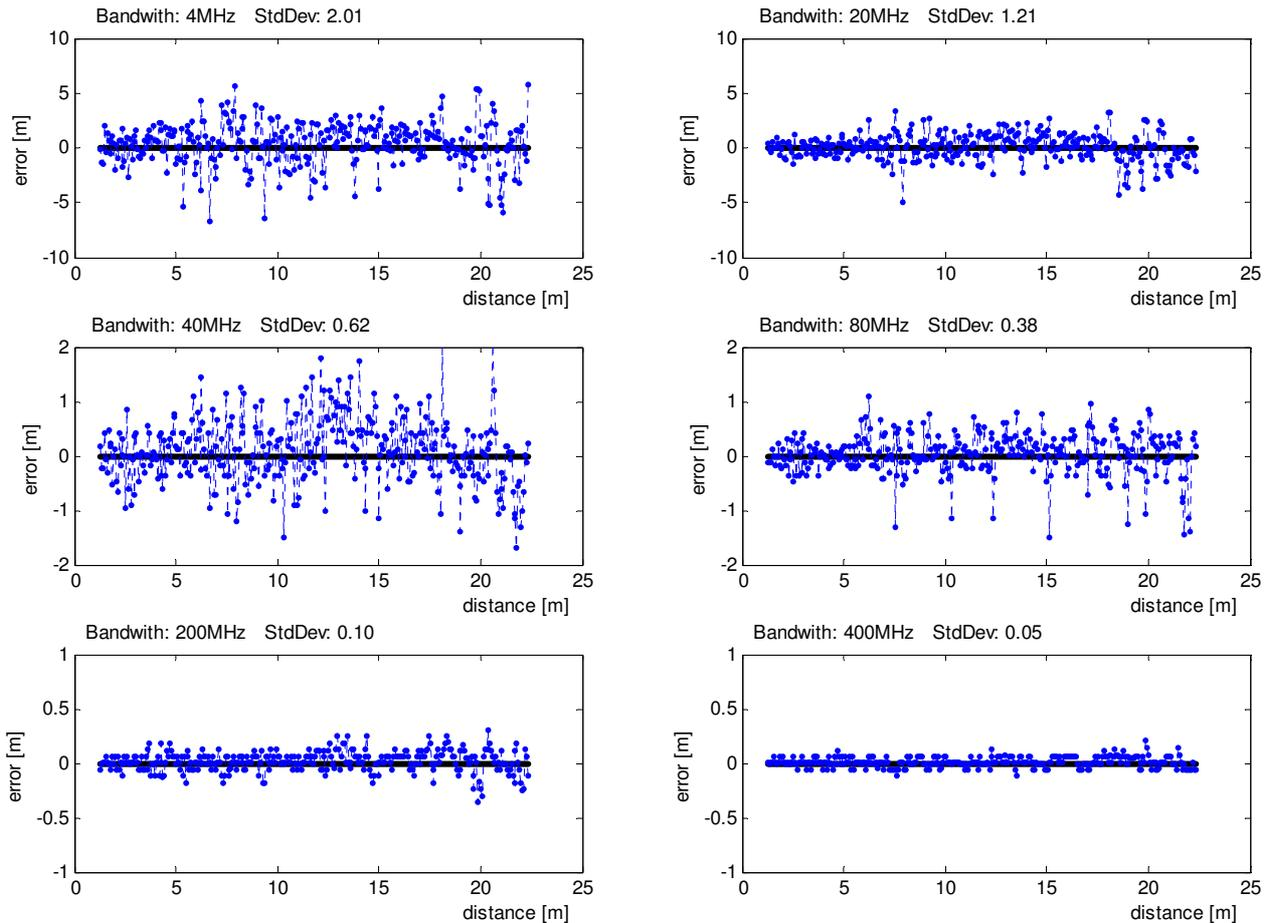
**Figure 74: Estimation error of the distance between car and VRU without an obstacle**
