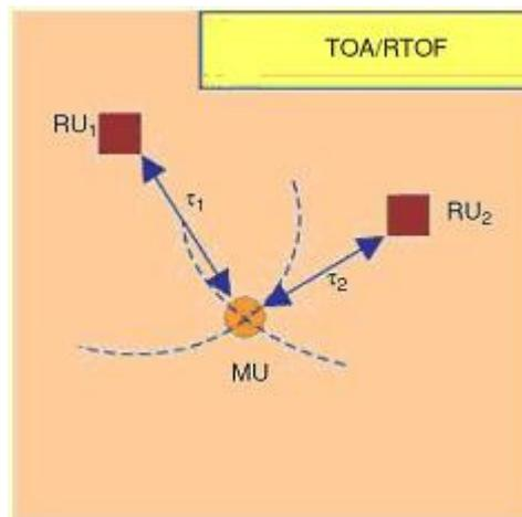
Figure 62: Measurement Principles for Time-of-Arrival (TOA) [16]
