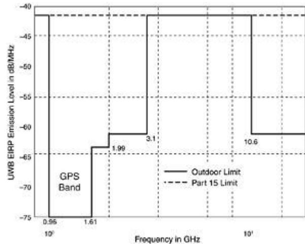
**Figure 50: UWB emission limits for outdoor communications systems [36]**
