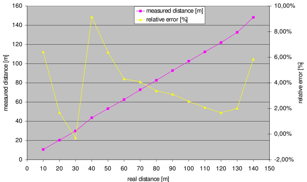
Fig. 23: Mean estimated distances and relative error for static measurements without obstacles in setup 2
