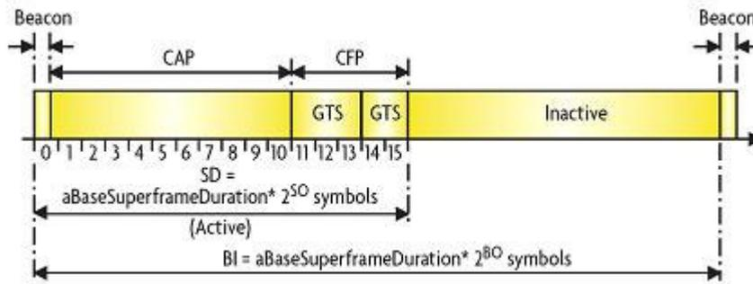
Figure 18: IEEE802.15.4 compatible beacon-enabled superframes
