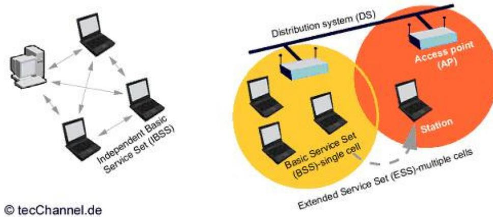
Figure 34: Architectures of the IEEE802.11 operation types [23]
