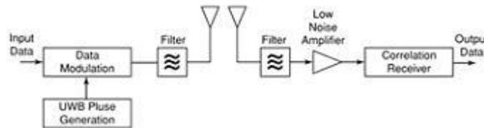
Figure 52: An example of an UWB transceiver architecture [36]
