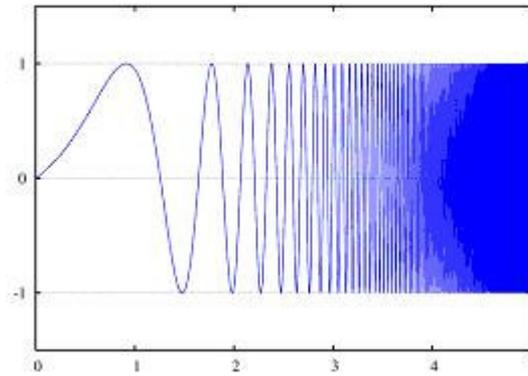
**Figure 22: An exponential chirp waveform**
