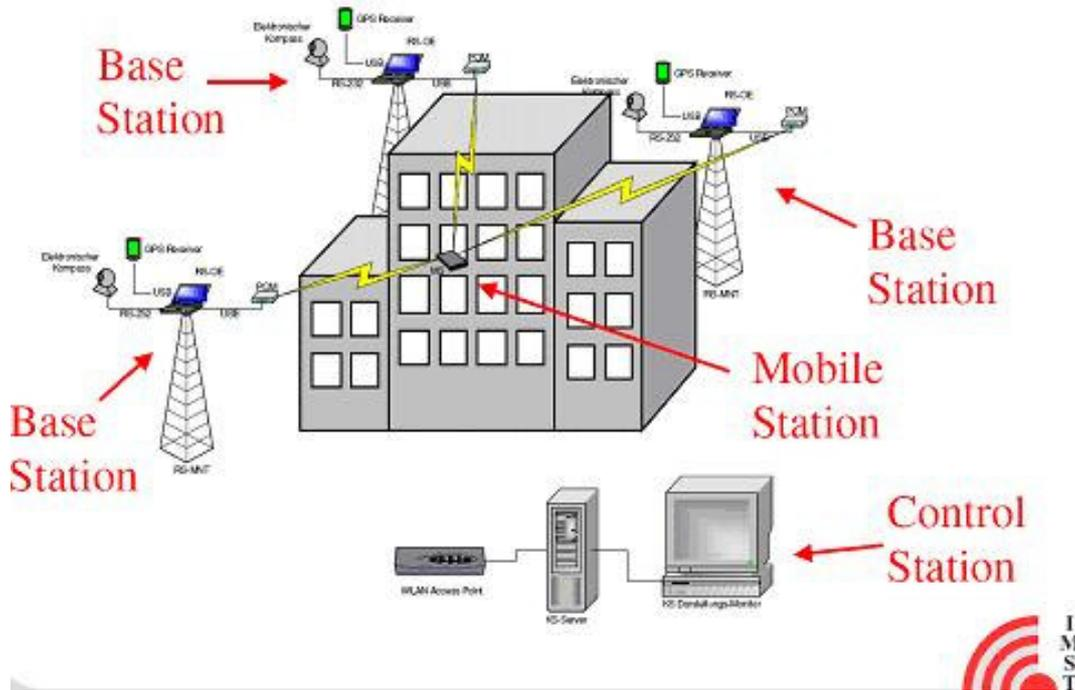
Figure 81: System architecture of Puls-On project [75]
