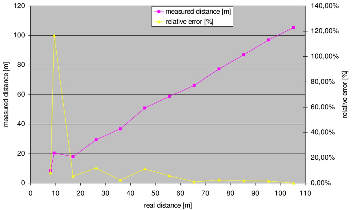
Fig. 25: Mean estimated distances and relative error for static measurements with obstacles in setup 2
