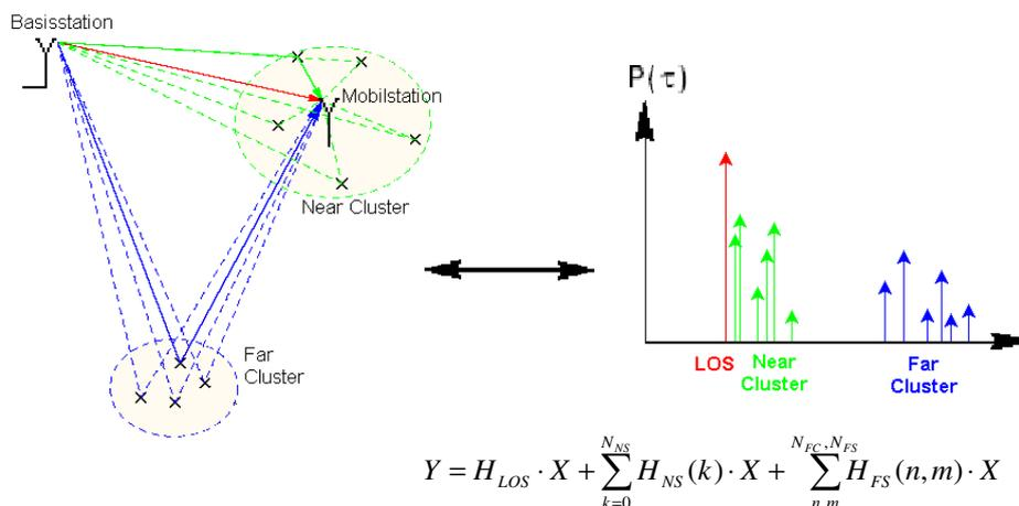
**Figure 72: geometrical situation with near and far cluster (left) and resulting power delay profile (right). The formula gives the superposition of several signals.**
