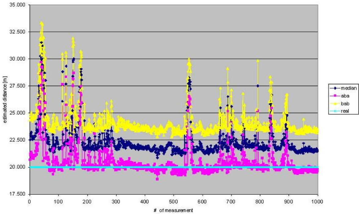
Fig. 16: Measurements with single deviating results; point a1, point b2 at a distance of 20 m with van at 15 m (raw results)
