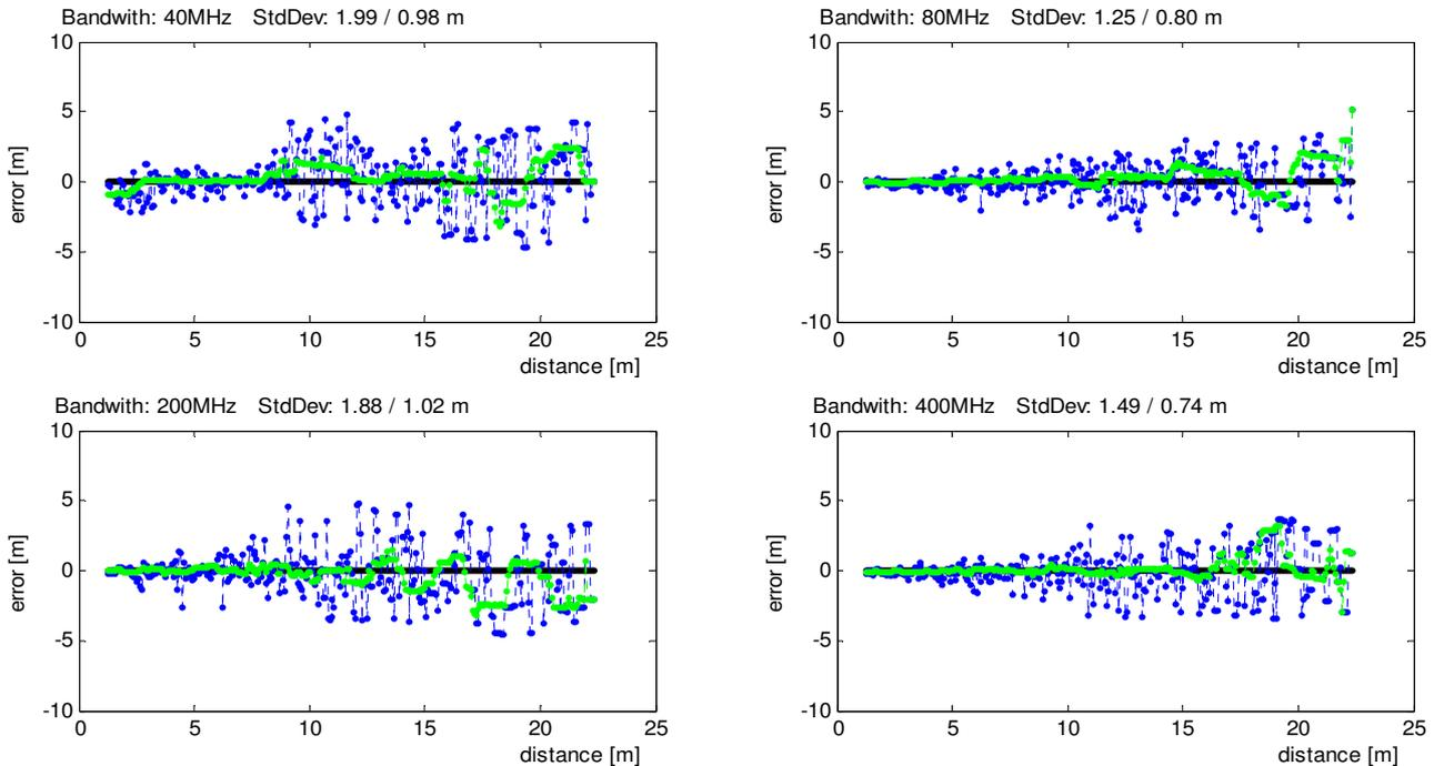
**Figure 80: Simulation results of the scenario depicted above with an obstacle. Parameters are BW 40-400MHz, SIR 2dB, SNR 0 – 20 dB. The green curve is the result of a post processing taking into account the trajectory of VRU.**
