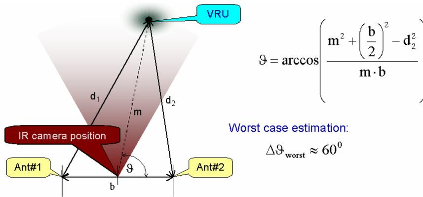
**Figure 4: Triangulation with two antennas for azimuth estimation**
