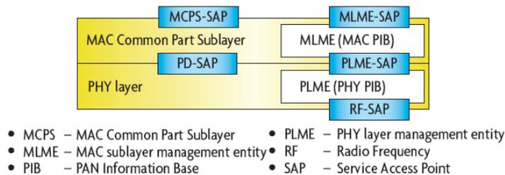
**Figure 14: Elements of the IEEE802.15.4 Protocol Stack**
