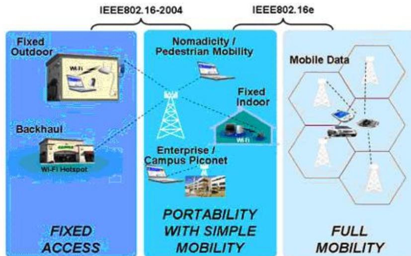
Figure 40: Architectures and Applications of IEEE802.16 (WiMAX) [30]
