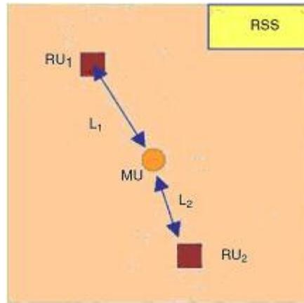
**Figure 60: Measurement Principles for Received Signal Strength (RSS) [16]**
