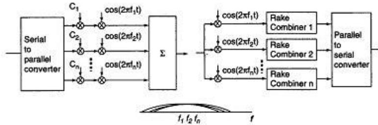
Figure 55: Block diagram and spectrum for multi-tone CDMA system [36]
