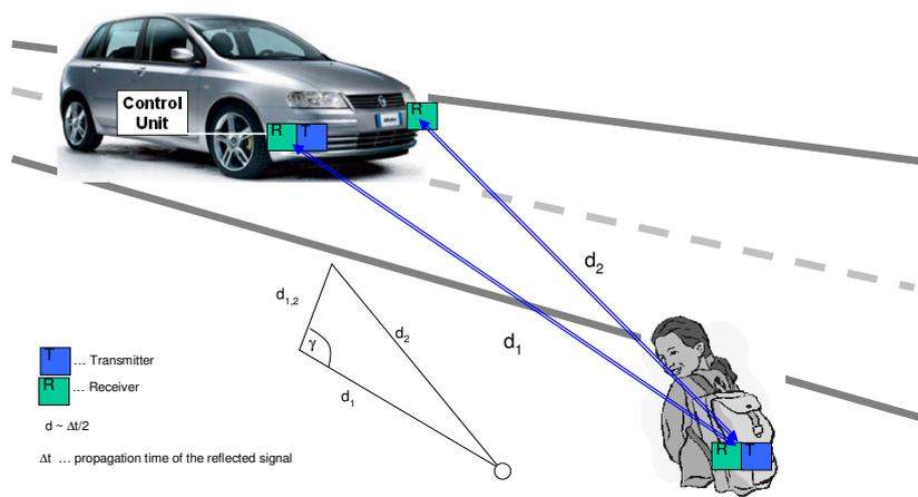
**Figure 68: Propagation time based approach with Roundtrip-Time-of-Flight (RTOF)**
