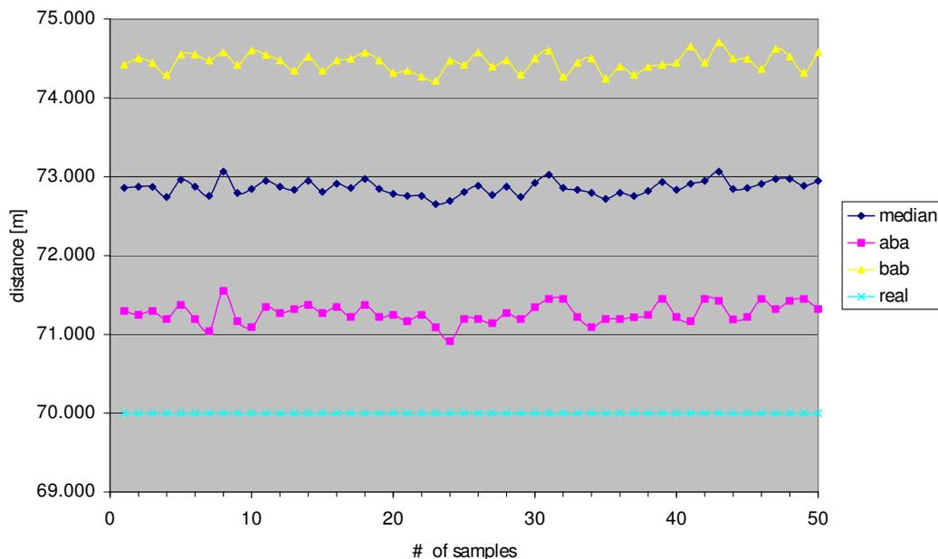
Fig. 22: Measurements with very homogeneous results; static measurement, no obstacles at a distance of 70 m
