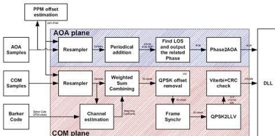
Figure 86: Internal architecture of Ittis base stations [75]
