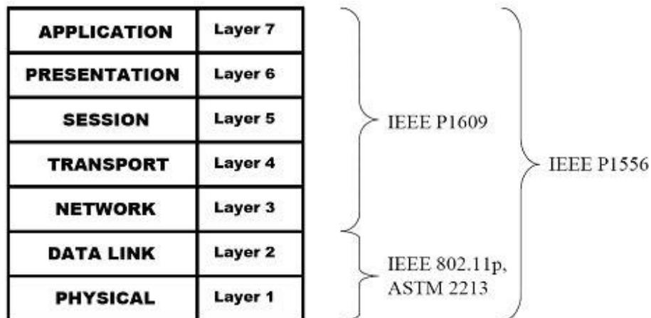
Figure 38: The elements of DSRC within the OSI reference model [29]
