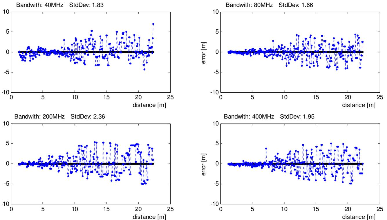
**Figure 79: Simulation results of the scenario depicted above with an obstacle. The simulation was done with different bandwidths (BW 40-400MHz) and a SIR of 2dB. The SNR depends on the distance and is in the range of 0 – 20 dB.**
