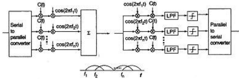
Figure 54: Block diagram and spectrum for multi-carrier DS-SS system [36]
