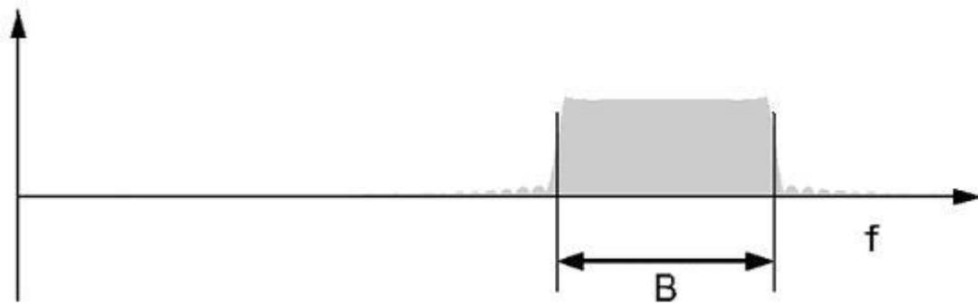
**Figure 21: The spectrum of the LFM pulse in the frequency domain**
