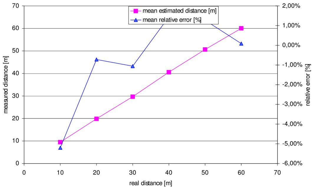
Fig. 31: Mean estimated distances and relative error for static measurements without obstacles in setup 2 using the nanoLOC ASIC
