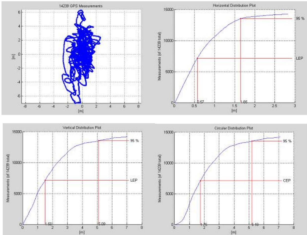
**Figure 87: Accuracy of results for self-localisation (measurement #1) static measurement scenario, good conditions)**
