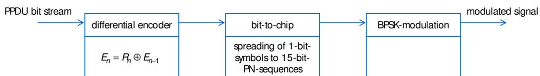
**Figure 16: Modulation Techniques for IEEE802.15.4 in the 900 MHz frequency band**
