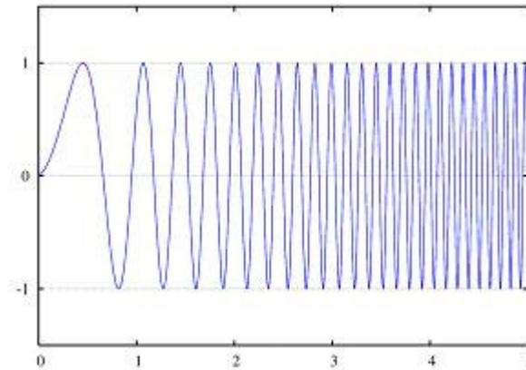
**Figure 20: A linear chirp waveform**
