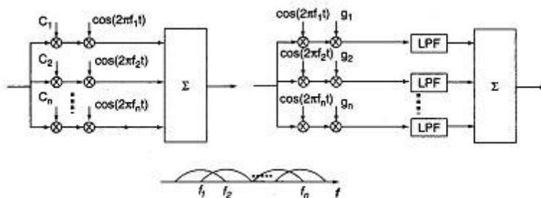
Figure 53: Block diagram and spectrum for multi-carrier CDMA system [36]
