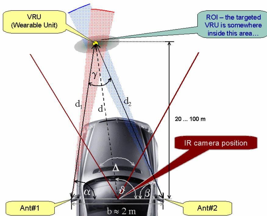
**Figure 3: Arrangement of the localisation system, angle measurement approach**
