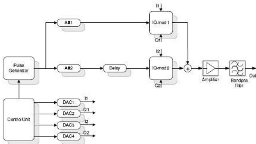
**Figure 83: Internal architecture of Iltis mobile stations [75]**
