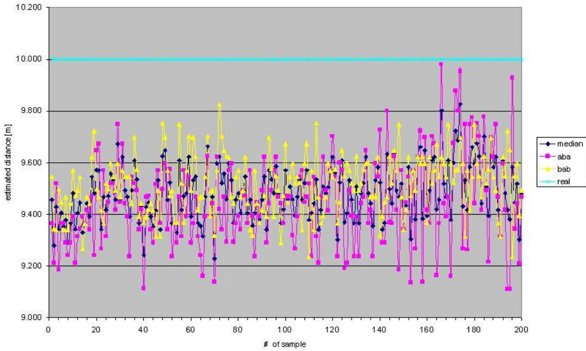
Fig. 29: Estimated distances for 200 samples using the nanoLOC ASIC; real distance is 10 m
