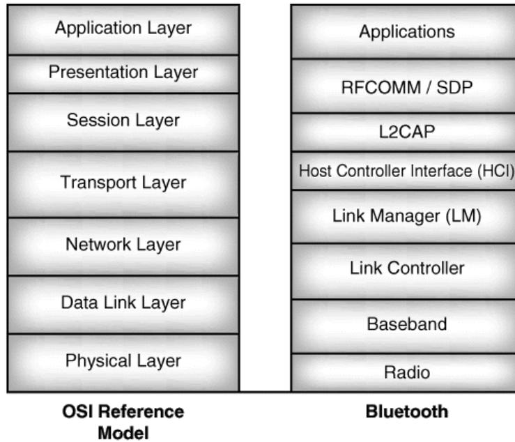
**Figure 28: The Bluetooth Stack in comparison to OSI Reference Model [24]**
