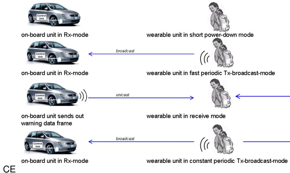
**Figure 11: Warning state of communication between wearable and on-board unit**
