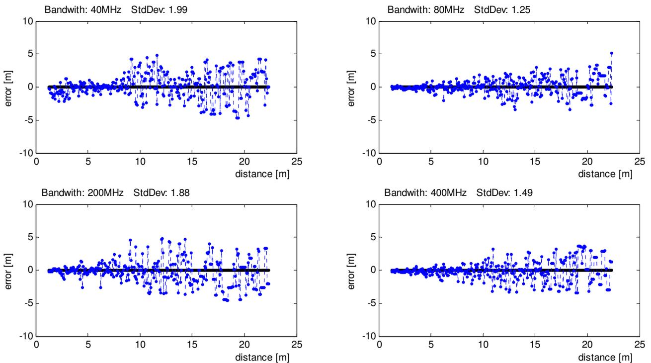
**Figure 78: Simulation results of the scenario depicted above without an obstacle. The simulation was done with different bandwidths (BW 40-400MHz) and a SIR of 2dB. The SNR depends on the distance and is in the range of 0 – 20 dB.**
