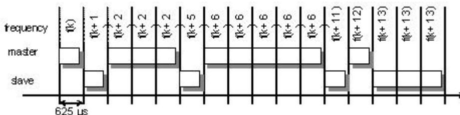
**Figure 29: Assignment of Bluetooth channels for single- and multislot-frames [23]**
