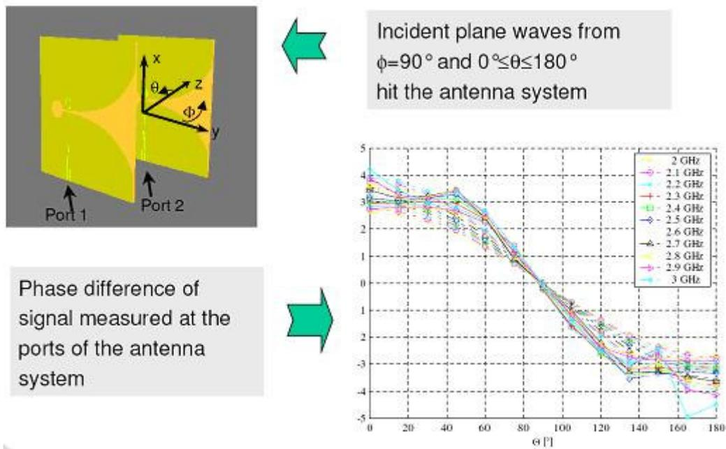
Figure 85: Determining the angle of arrival in an Ittis base station from IMST [75]
