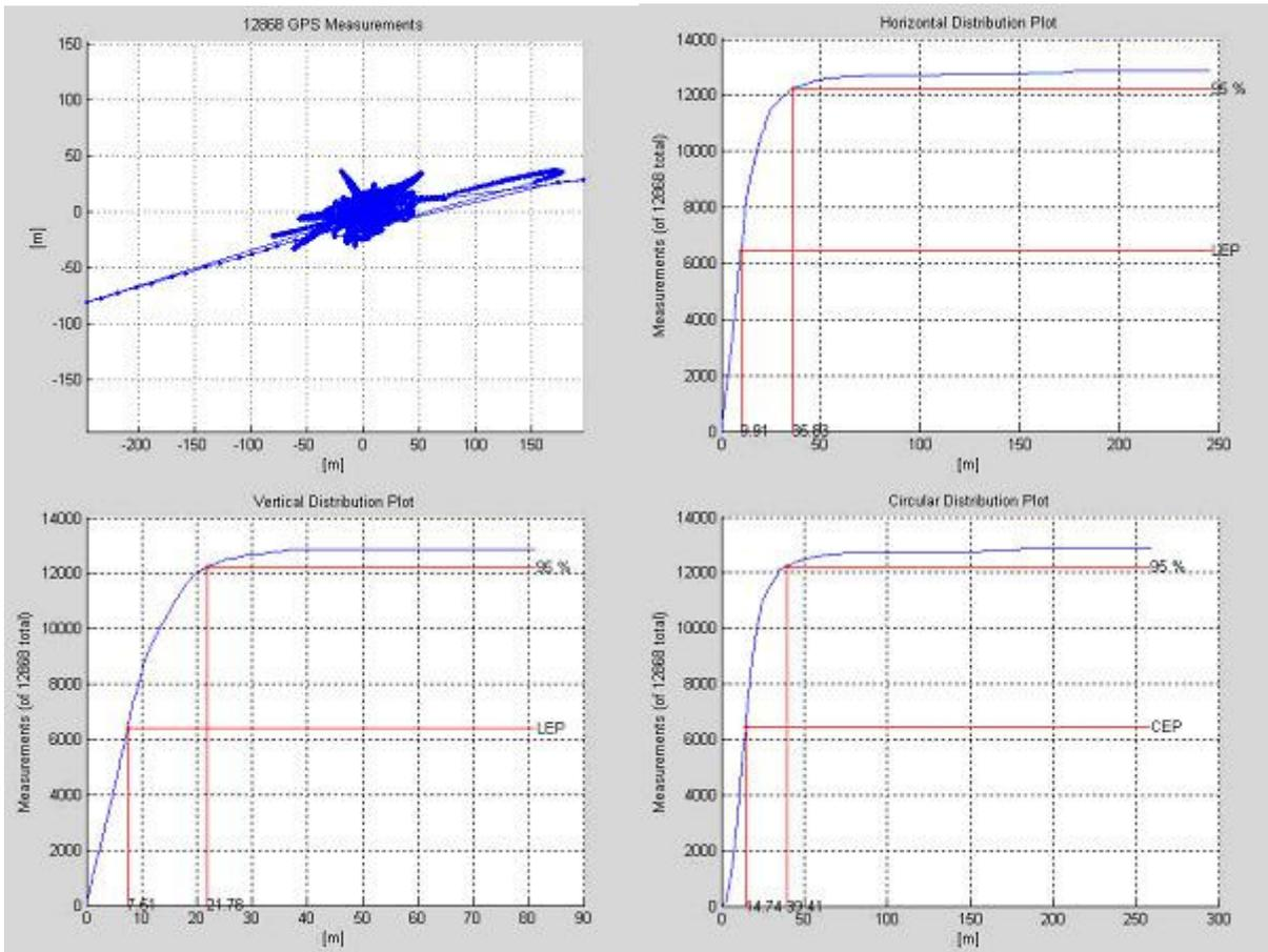
**Figure 88: Accuracy of results for self-localisation (measurement #2) static measurement scenario, bad conditions)**
