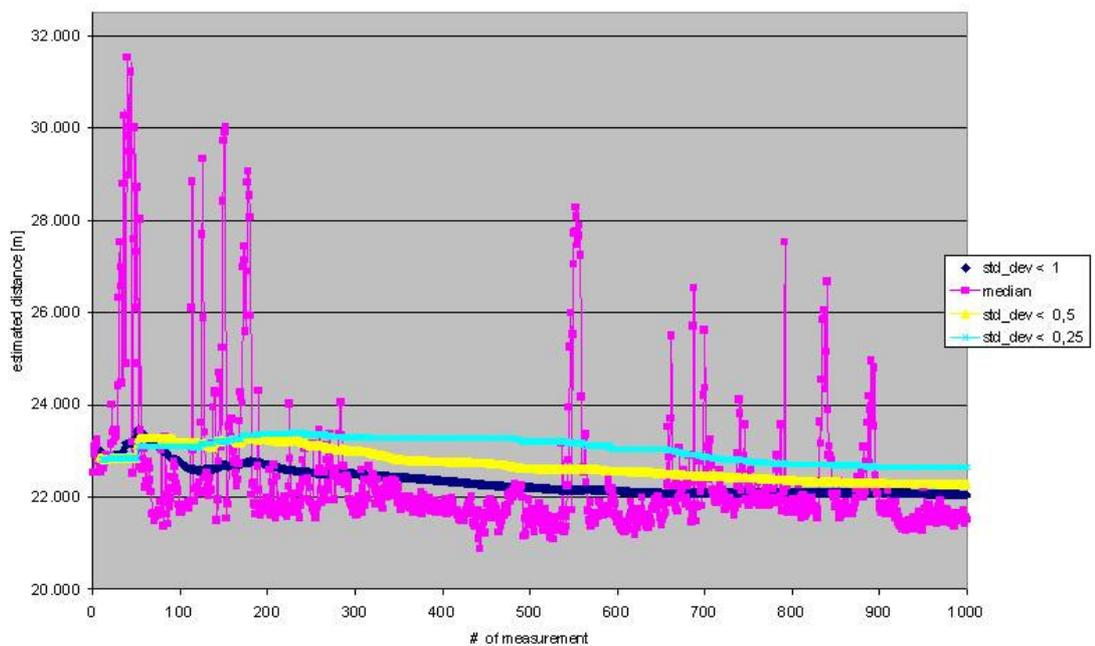
Fig. 17: Mean values excluding results with too large a deviation; mean values and standard deviation are calculated on a flowing basis
