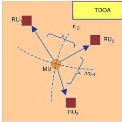
**Figure 63: Measurement Principles for Time-Difference-of-Arrival (TDOA) [16]**
