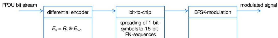
**Figure 15: Modulation Techniques for IEEE802.15.4 in the 2.4 GHz frequency band**
