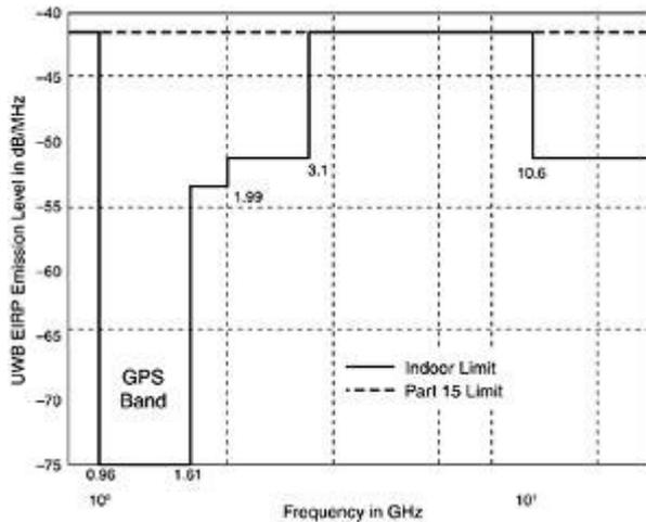
**Figure 49: UWB emission limits for indoor communications systems [36]**
