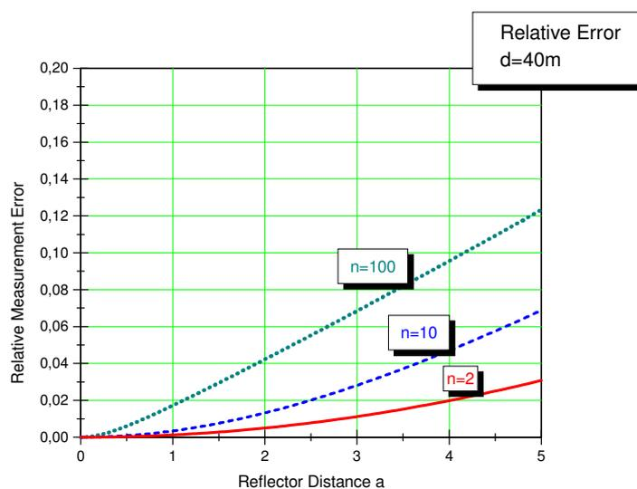
**Figure 7: Relative NLOS Measurement Error for  $d = 40$  m**
