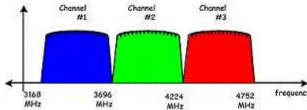
Figure 56: Frequency allocation of sub-bands for a multi-band OFDM system [33]
