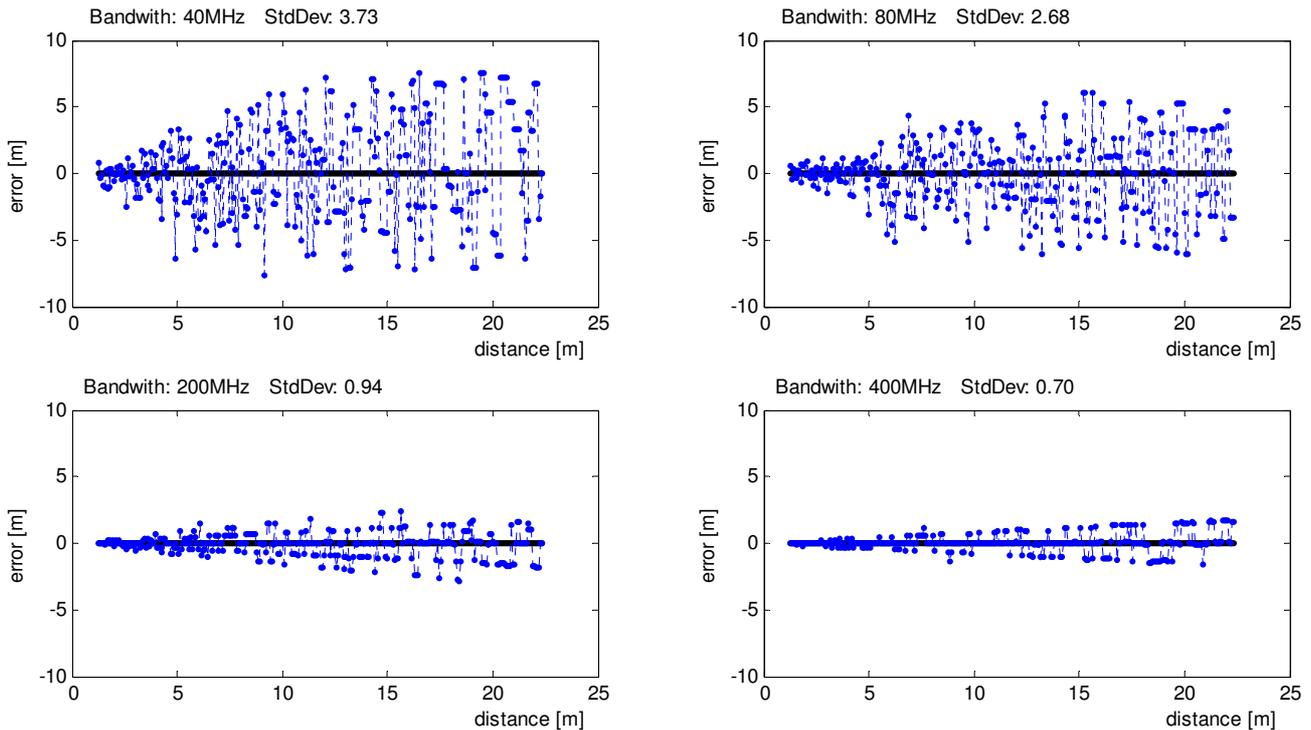
**Figure 76: Estimation error of the VRU position relative to the road using triangulation without an obstacle**
