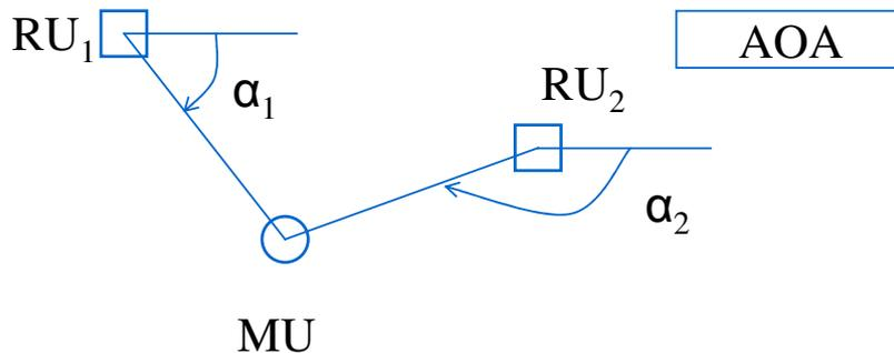
**Figure 61: Measurement Principles for Angle-of-Arrival (AOA) [16]**
