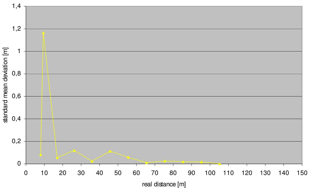
Fig. 26: Standard mean deviation for static measurements with obstacles in setup 2
