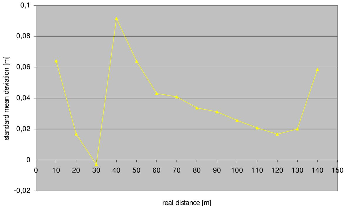
Fig. 24: Standard mean deviation for static measurements without obstacles in setup 2
