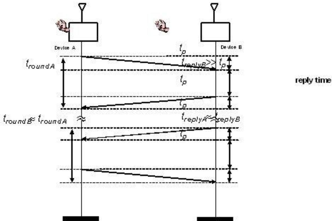
Figure 67: Symmetric Double Sided Two Way Ranging [21]
