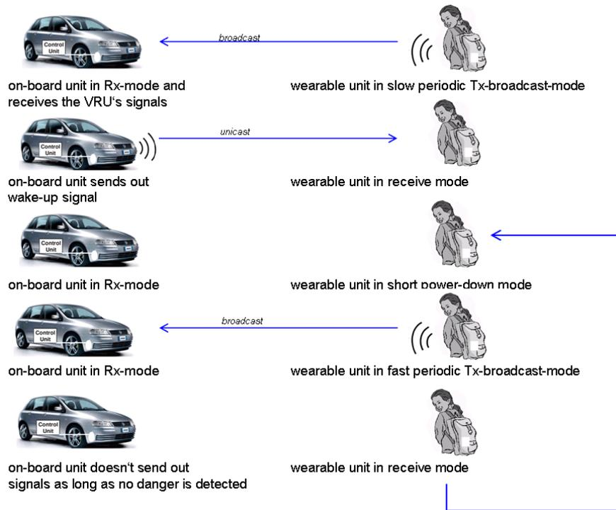
**Figure 10: Detected state of communication between wearable and on-board unit**
