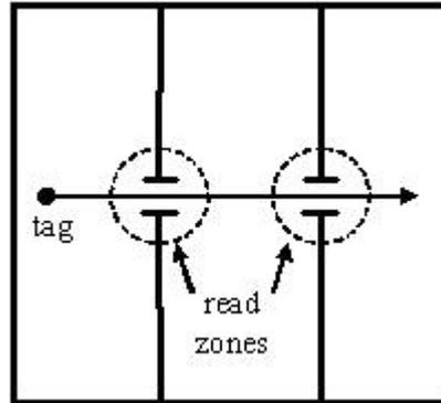
**Figure 46: Non-overlapping read zones with choke-points**
