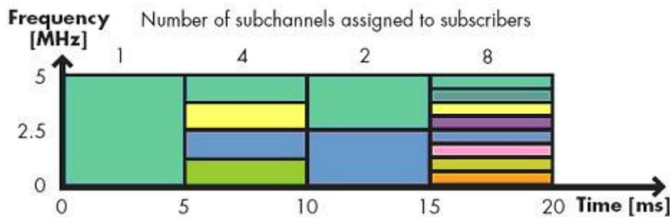
**Figure 41: Scalable OFDMA: dynamic assignment of subcarriers to subscribers [61]**
