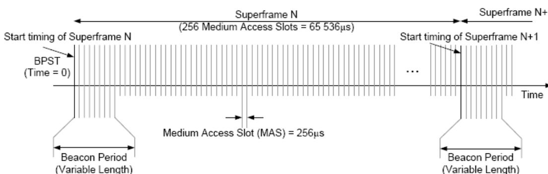
**Figure 58: UWB MAC superframe structure according to ECMA-368 [73]**
