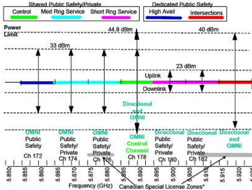
**Figure 39: Frequency channel and antenna plan for IEEE802.11p in the FCC regions [30]**
