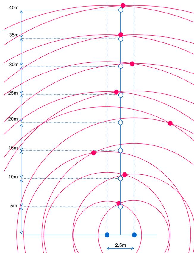
Fig. 11: Illustration of measurement results for test setup 1 without obstacles. The circles show the diameter of the measured distances from both points a1 and a3.
