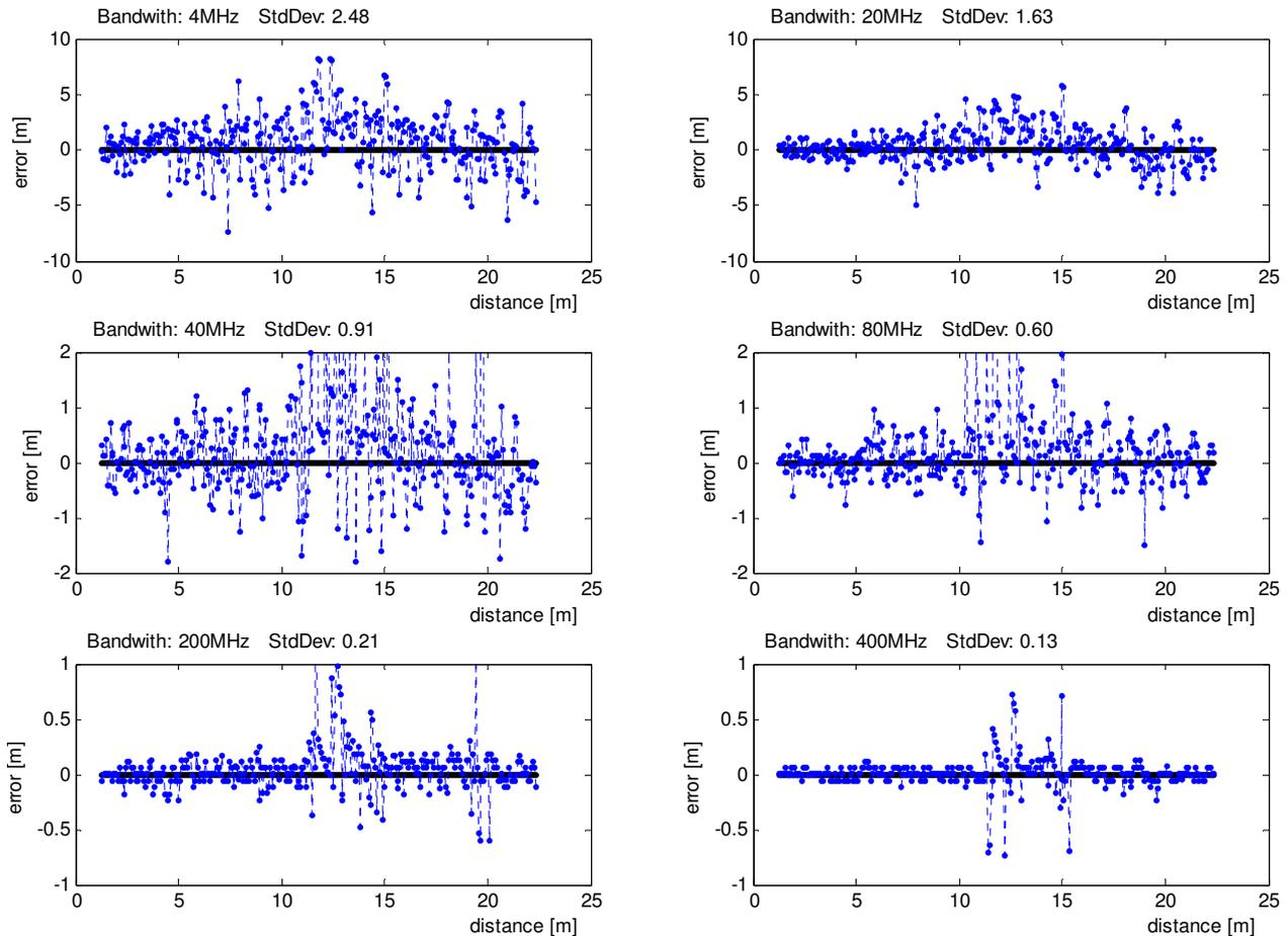
**Figure 75: Estimation error of the distance between car and VRU with an obstacle**
