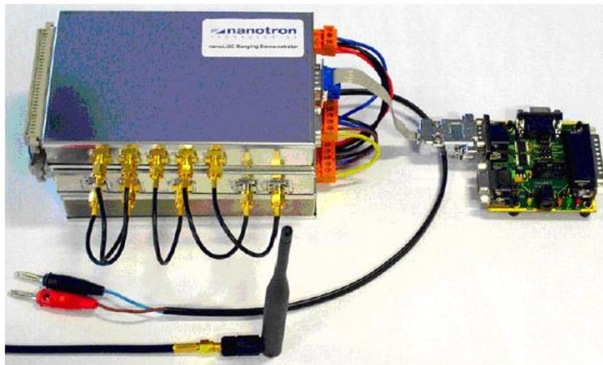
Fig. 1: nanoLOC DHP Ranging Demonstrator components
