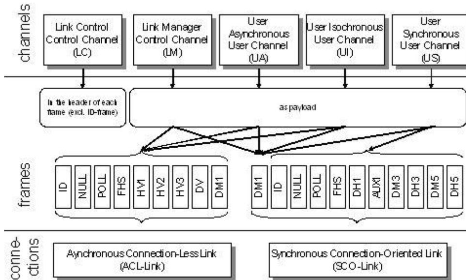
Figure 30: Assignment of Bluetooth channels to frame formats and connections [23]
