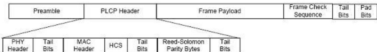
Figure 57: UWB PHY frame structure according to ECMA-368 [73]
