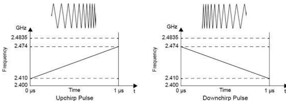
**Figure 25: Upchirp and Downchirp pulses in time domain [85]**
